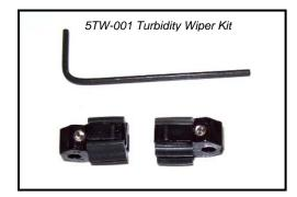
To change the wiper, loosen the set screw in the wiper arm until the wiper assembly can be removed from the wiping shaft. Place a new wiper assembly on the shaft with the set screw aligned squarely with the flat on the wiping shaft. Gently press the wiper arm down until the wiper arm hits the stop on the shaft. The wiper pad should now be compressed to roughly one half its original thickness. Tighten the set screw do not over tighten.
